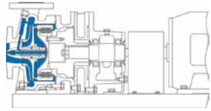
Bearing frame mounted MKP OH2 HT (high temperature) with centreline support -148 to +662°F
