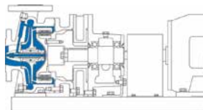
Bearing frame mounted MKP OH2 HT (high temperature) with centreline support -100 to +350°C
