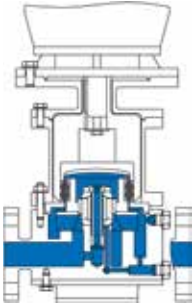
Vertical in-line close-coupled SZMK with stand -100°C to +200°C
